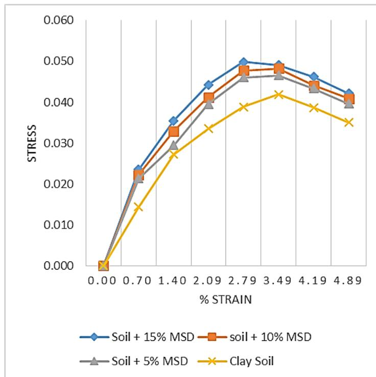
Figure 17. Overall comparison of all strain vs. stress graphs for all samples in UCS
