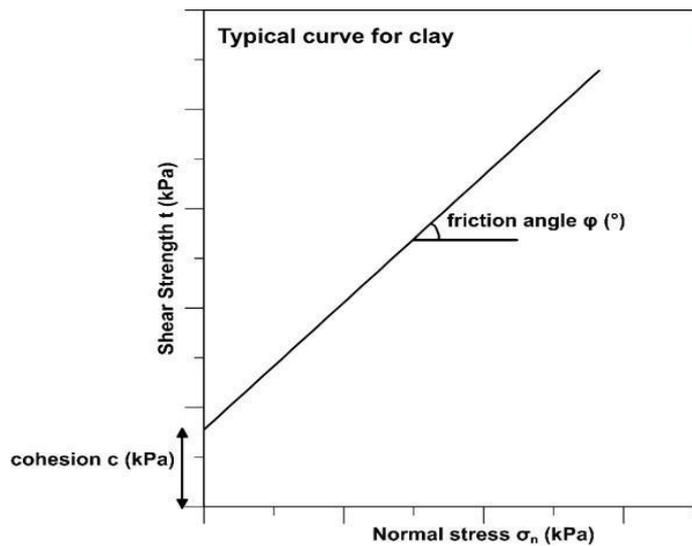
**Figure SEQ Figure \\* ARABIC 1 The cohesion ( $c$ ) and angle of internal friction ( $\phi$ )**
