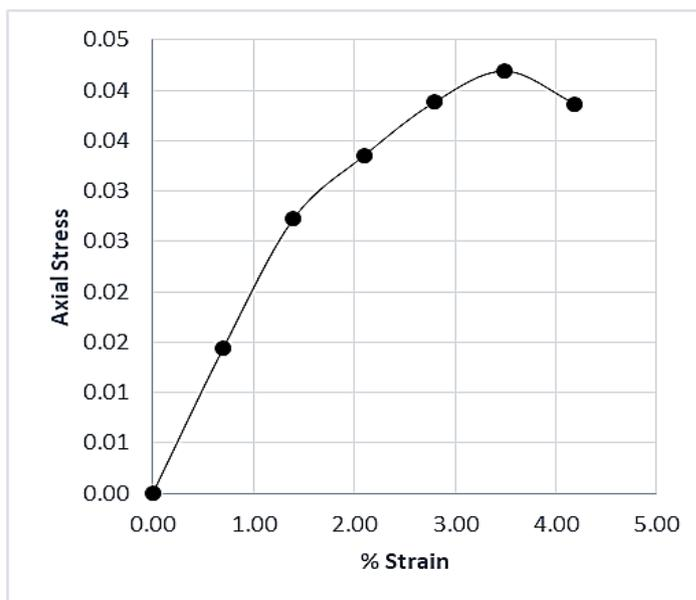
**Figure 13. Strain vs. Stress graph for clay soil**
