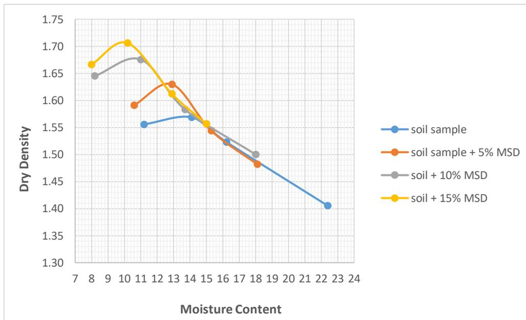
Figure 12. Overall comparison between OMC and MDD of all tested sample
