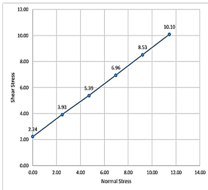
Figure SEQ Figure \\* ARABIC 3 shear stress vs normal stress for clay soil + 5% MSD in direct shear test
