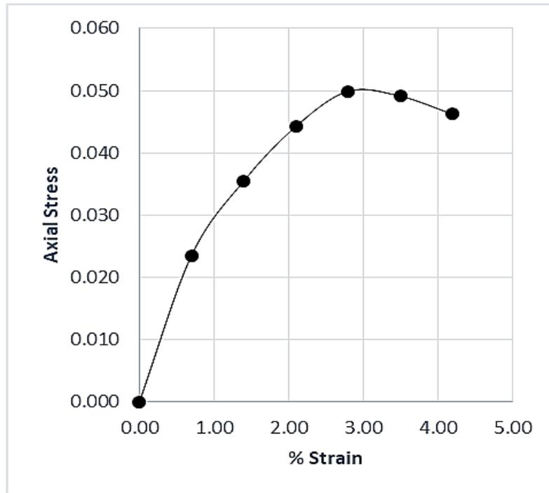
Figure 16. Strain vs. Stress graph for clay soil+15% MSD in UCS
