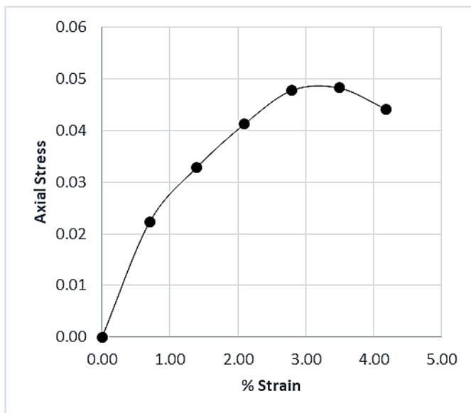
Figure 15. Strain vs. Stress graph for clay soil+10% MSD in UCS
