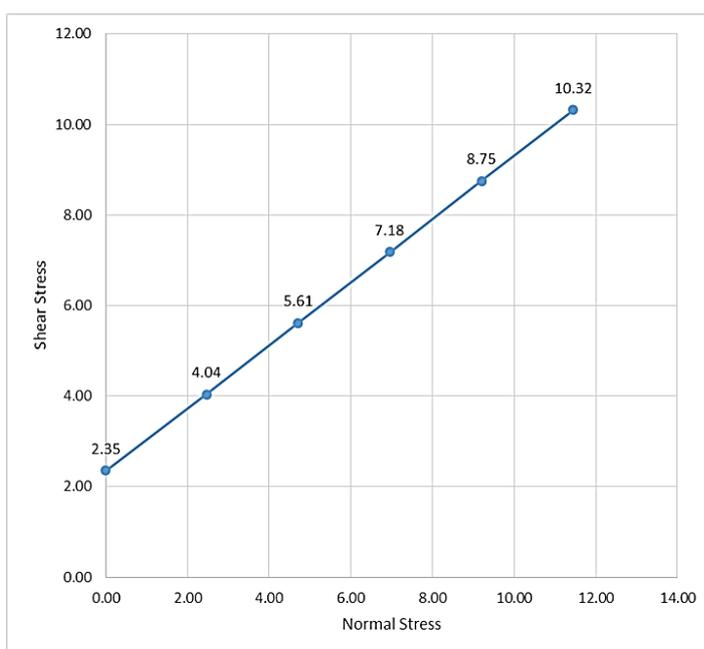
Figure SEQ Figure \\* ARABIC 4 Shear stress vs normal stress for clay soil + 10% MSD in direct shear stress
