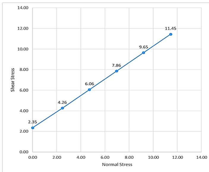
Figure SEQ Figure \\* ARABIC 5 shear stress vs. normal stress for clay soil+15% MSD in direct shear test
