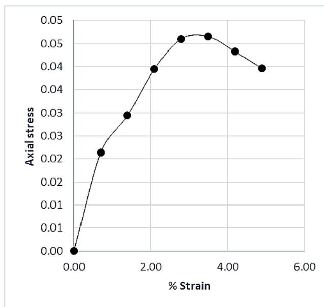
**Figure 14. Strain vs. Stress graph for clay soil+5% MSD in UCS**
