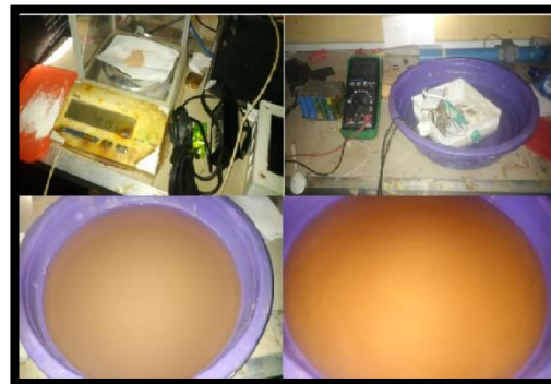
Plate 4: Laboratory Calibration of Turbidity Sensor at Physics Department FUTA for the WSSV
