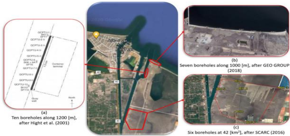
Figure 3 Location’s map showing the executed boreholes at East Port-Said (after Tolba et al., 2020)
